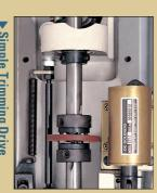
Simple Trimming Drive Devices(Trimming Type) It is easy to set up the gauge transformation by adjusting the length of rod.
